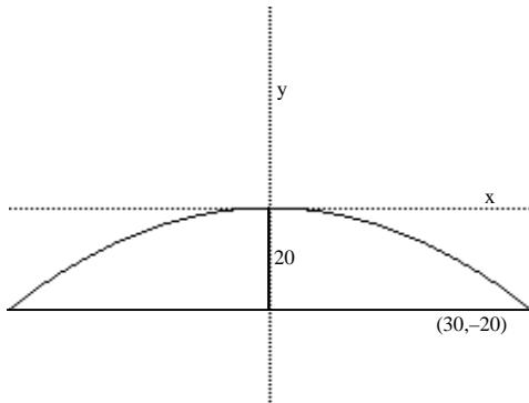
To find the height of the bridge, 5 feet from the center, the point  $(5, y)$  is a point on the parabola.
