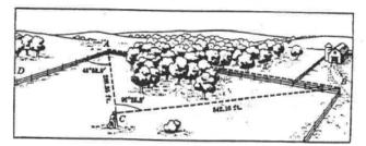
chosen in the field 286.35 feet from A and 342.16 feet from B, and the angle ACB is measured as 96°25.8′. Find the length of AB. Also, if the angle DAC is measured as 48°53.9′, find the angle DAB.
